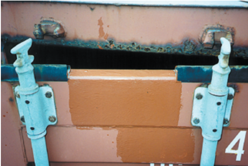
Photo 10.9 (to right) / Gasket section installed (exterior view)
