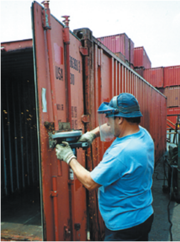
Photo 10.1 / Cutting locking bar with a disc cutter
