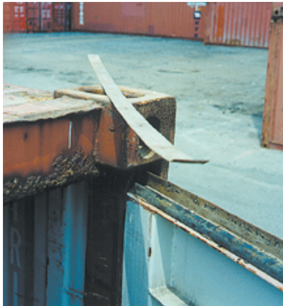
Photo 10.6 (to left) / Removed gasket retaining strip
