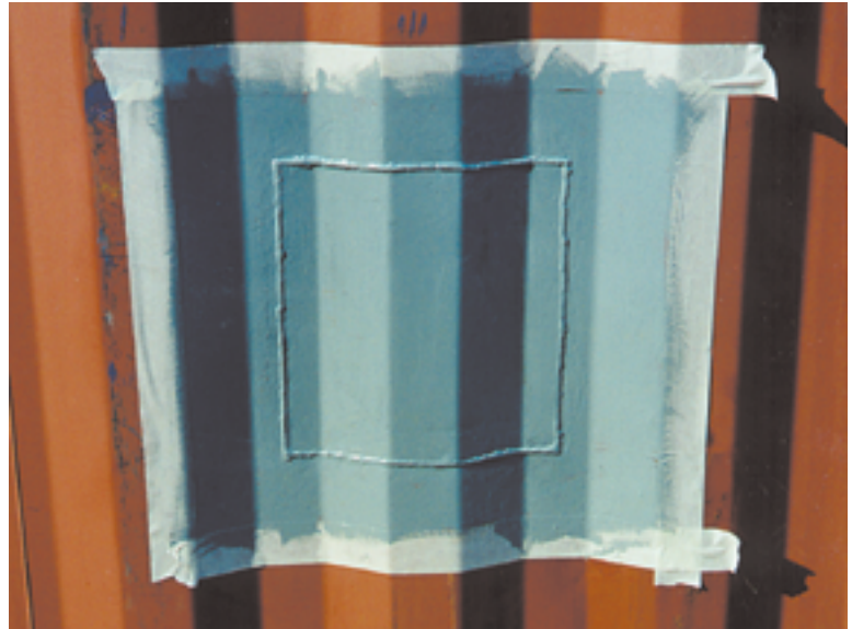
Photo 2.10 (to right) / Masking and priming of panel insert repair
