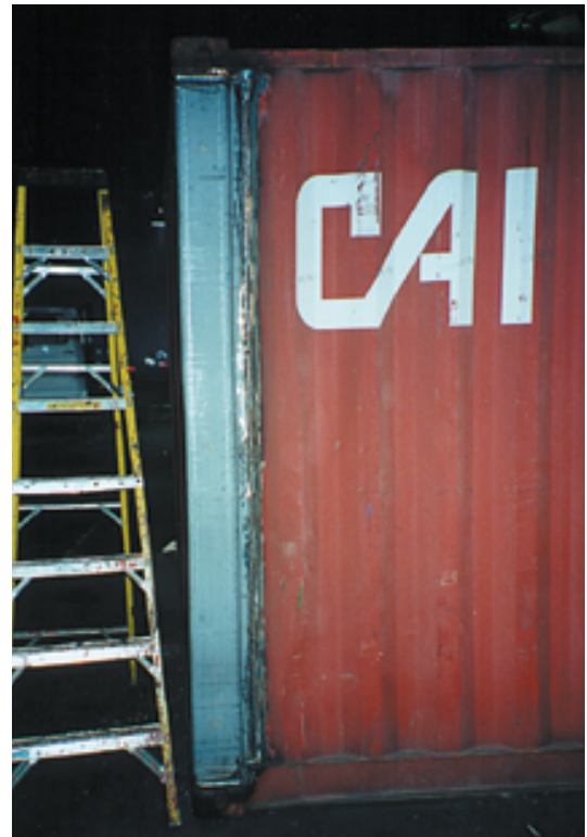
Photo 2.26 (below) / Detail of front corner post welding adjacent to corner fitting
