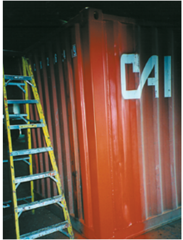
Photo 2.29 / Top coating of replacement front corner post (exterior)
