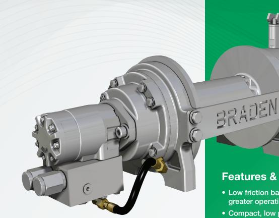
TR Series planetary winches are designed for standalone use on trailers, as well as towing and self-recovery applications. The highly efficient and rugged design of the gear train allows for fast line speeds and continuous winch operation. With versatile mounting options and line pull ratings from 12,000 lb (5,443 kg) to 30,000 lb (13,608 kg), TR Series winches are easily adaptable to multiple applications.
